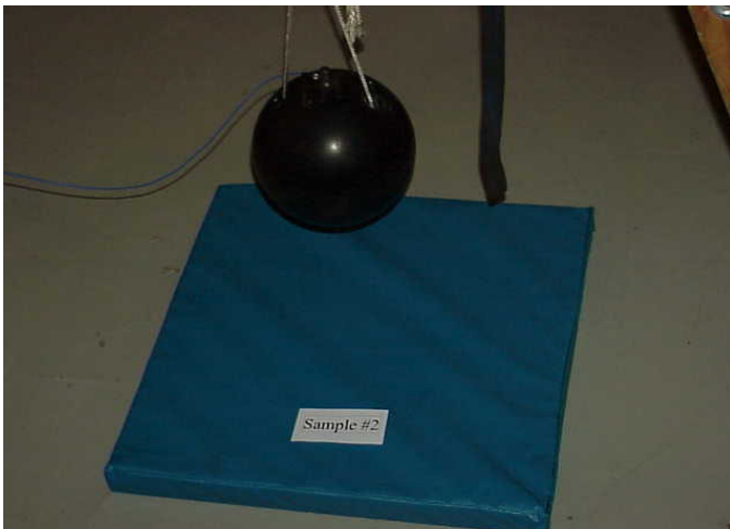
Drop test (representative). Sample No. 3.
