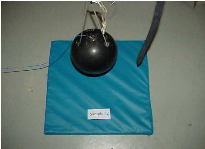
Drop test (representative). Sample No. 2.
